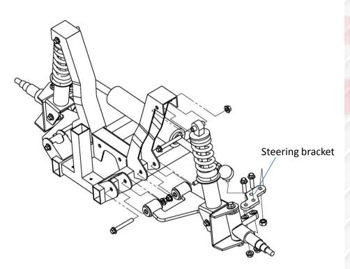
1. Remove front wheels and hubs. Then disconnect tie rod end from spindles, shock from cart frame, a-arm from cart frame. Try to take off spindle, knuckle bracket and a-arm as a whole assembly. Discard steering bracket.
