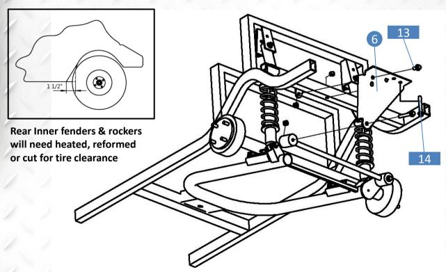
13. Attach sway bar bracket #6 using hardware #13, M10-90 from hardware #14 through the drilled hole down to top. Attach sway bar to sway bar bracket using factory hardware. Install larger wheels on.
