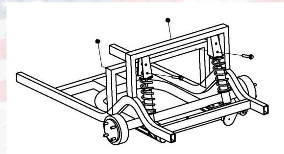
10. Remove motor cover and retain. Remove upper bolt from rear shocks on both sides. Retain hardware.
