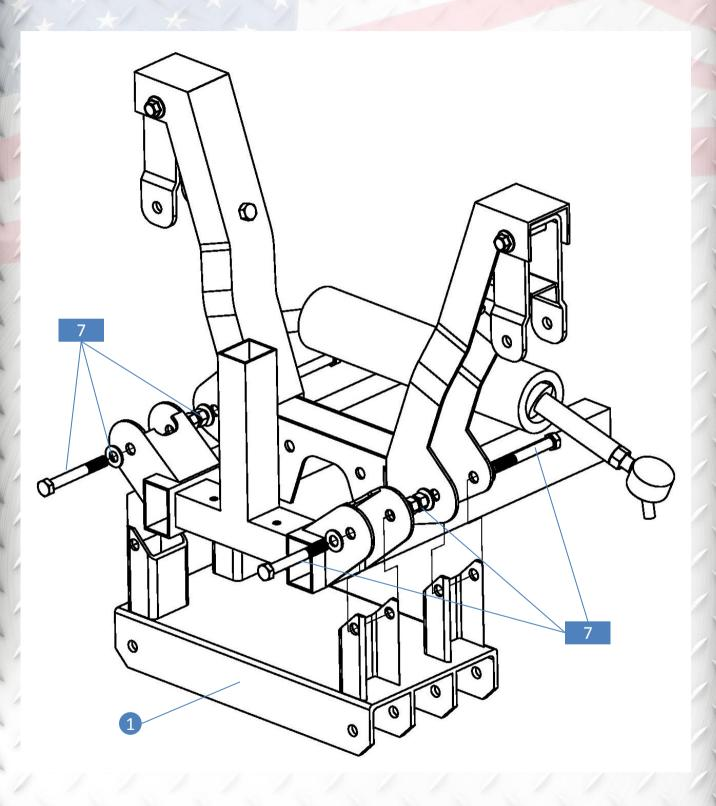
5. Install main bracket #1 on the cart using hardware #7.
