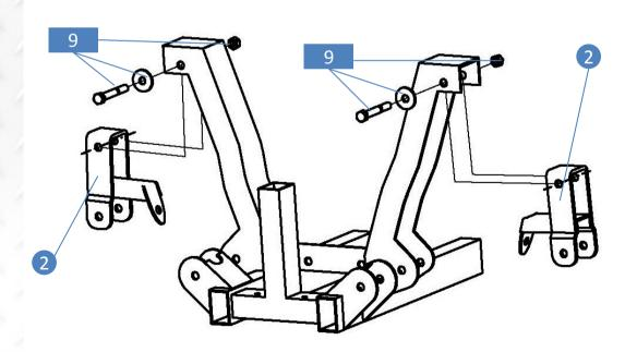
2. Install front shock mounting bracket #2 on the cart frame using supplied Hardware #9.
