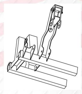
3. Rotate the front shock mounting bracket #2 so the lower proportion of it leans on the cart frame.
