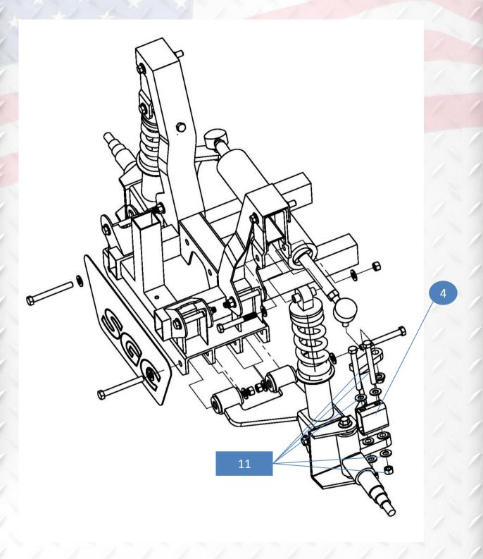
6. Install steering riser #4 on factory spindle using hardware #11.
