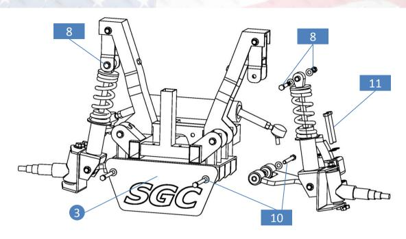
7. Attach SGC plate #3 to main bracket. Attach a-arm to main bracket with hardware #10. Attach shock to shock mounting bracket with hardware #8. Attach tie rod end to steering riser with retained hardware.
