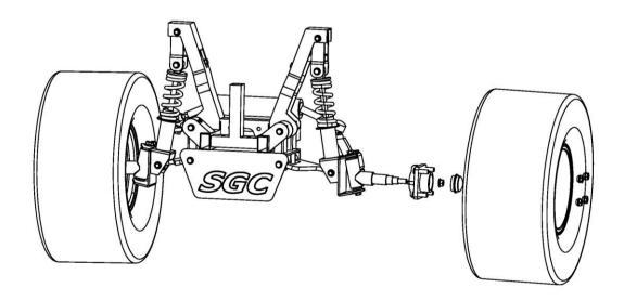
8. Reinstall hubs and install new large front wheels.
