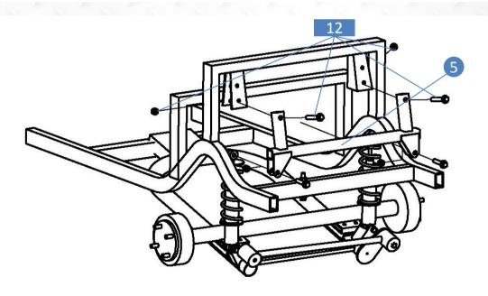
11. Attach rear mounting bracket #5 in the opening using hardware #12. Be sure the ends of the bracket are angled towards the front of the cart. Attach upper portion of rear shock to rear mounting bracket using hardware from step 10.
