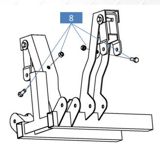
4. Use a marker pencil to locate the hole on the cart frame, drill it with provided drill bit #15. Then secure the front shock mounting bracket on the cart frame with hardware #8.
