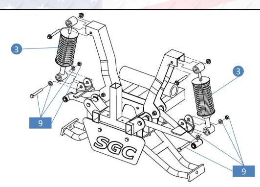
6. Attach coilover shock #3 to cart frame using retained hardware and to upper a-arm #2 using supplied hardware #9.
