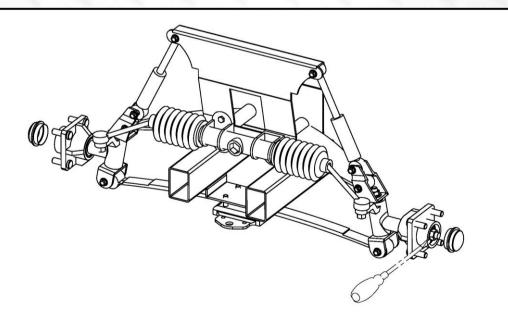
2. Remove dust cover, cotter pin and hub. Retain hardware.
