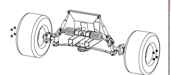
1. Engage park brake. Raise cart with lift and support with jack stands. Remove front wheels. Remove front bumper. Retain hardware.
