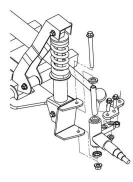
3. Remove spindle from knuckle bracket.
