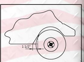
Rear Inner fenders & rockers will need heated, reformed or cut for tire clearance
