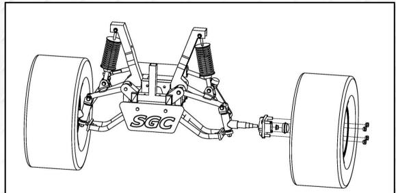
9. Reattach hubs and larger wheels. Front installation completed.
