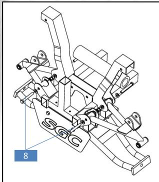
5. Attach main suspension assembly #1 to cart frame. Align the holes but don't bolt on.
