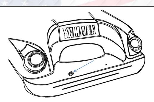
12. Drill hole through the bagwell in the location shown. Depending on manufacturing year, a rivet or bolt should be removed first. Be sure to drill straight down through entire frame. Drill bit provided.
