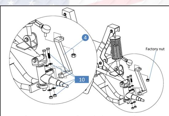
8. Install steering riser #4 to spindle using hardware #10. Attach steering riser to tie rod end using factory nut.
