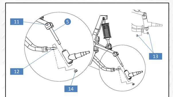
7. Install heim joint #12 on the lower a-arm using supplied hex nuts 1/2. Then install the kingpin #5 on the upper a-arm #2 using hardware #11. Attach factory spindle to the kingpin then secure end of kingpin to heim joint using supplied nut M12.
