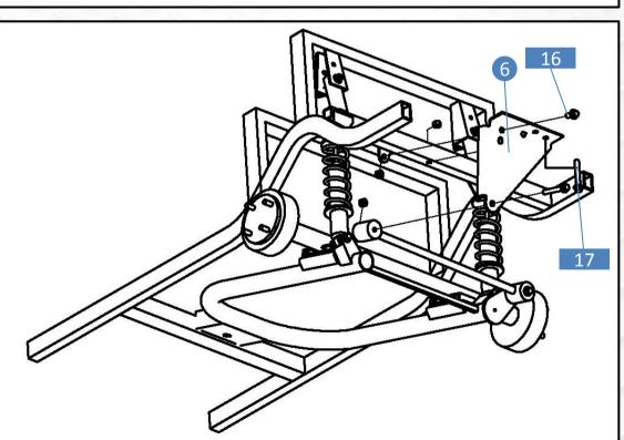
13. Attach sway bar bracket #6 using hardware #16, then M10-90 from hardware #17 from the drilled hole down to top. Attach sway bar to sway bar bracket using factory hardware.
