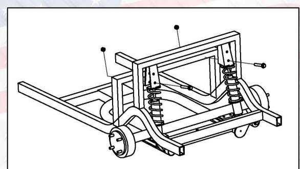
10. Remove motor cover and retain. Remove upper bolt from rear shocks on both sides. Retain hardware.
