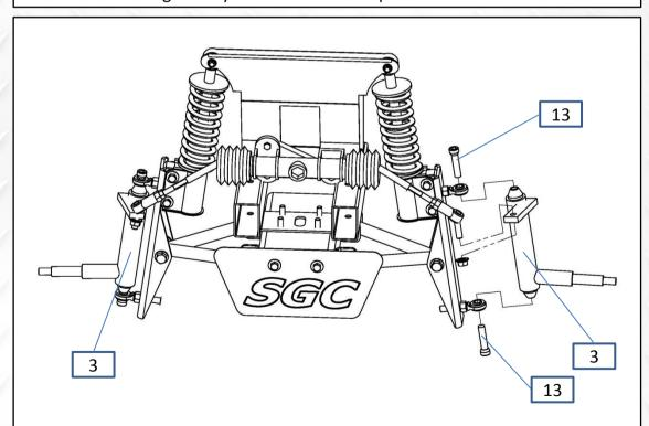
10. Install supplied spindle #3 on heim joint using supplied egg neck bolt #13. Attach tie-rod end to spindle using factory hardware.
