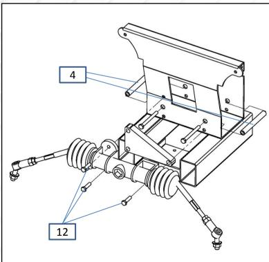
6. Reinstall rack and pinion and supplied spacer to cart frame using supplied hardware #12.
