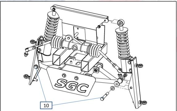
9. Attach spindle bracket #2 to upper a-arm from main suspension frame using supplied hardware #10 (detached in step 7). Attach top of shock absorber #5 to cart frame using factory hardware from step3.
