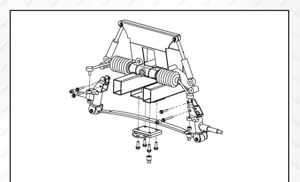
4. Using 1/2" socket remove factory spindle. Using a 1/2" socket remove spring plate and leaf spring.
