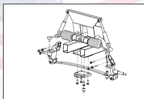
3. Using a 1/2" socket remove bolt from shock and retain. Push shock up and out of the way. Remove and retain the cotter pin from tie rod end, using an 18mm socket and 11/16" wrench. Remove nut from tie rod and retain.
