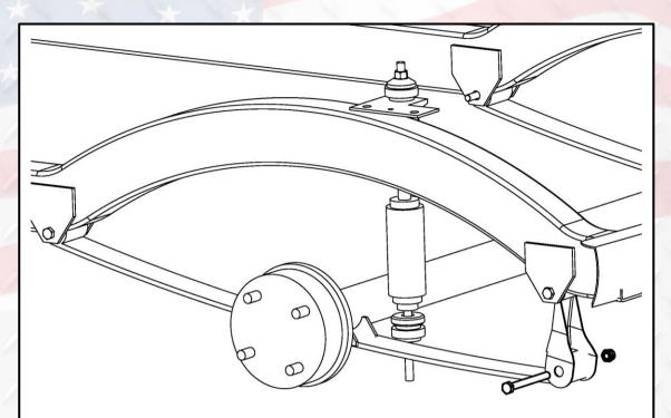
14. Using a 10mm socket and 13mm wrench remove hardware from rear leaf spring mount and front leaf spring mount. Retain hardware.
