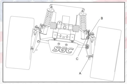
**IMPORTANT:** Both Camber and Toe must be adjusted on this model.
