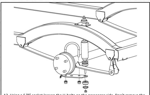
13. Using a 5/8" socket loosen the U-bolts on the passenger side. Don't remove the U-bolts. It's important to do one side at a time to avoid motor roll. Loosening but not removing the U-bolts will make this easier.
