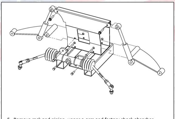
5. Remove rack and pinion, upper a-arm and factory shock absorber.
