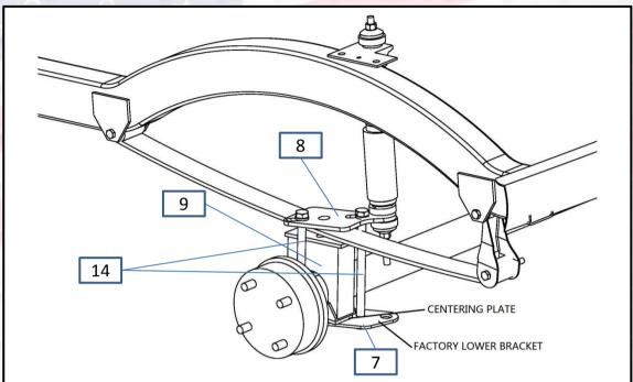
14. Route supplied bolts M12\*180 through shock plate #8, rear lift block #9 and factory lower bracket making sure centering plate #7 fits properly. Using socket to tighten these four bolts evenly to ensure proper alignment.
